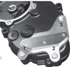
1) Remove the three bolts from the OEM cover as shown in the diagram at the right.
